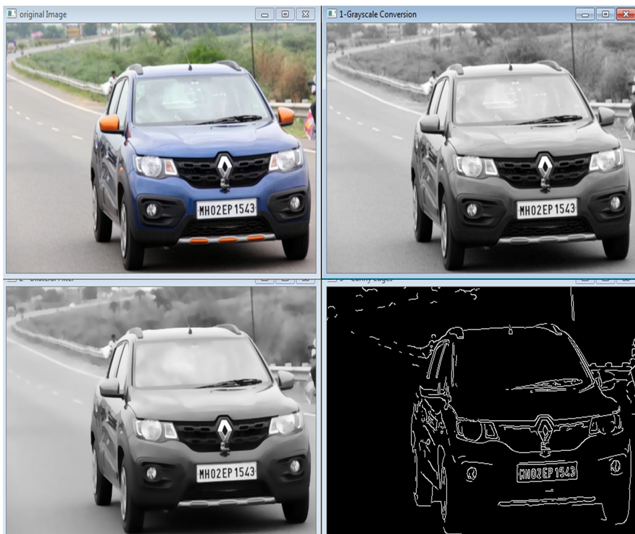
Figure 2: Automatic Number Plate Recognition system acquiring the number plate
