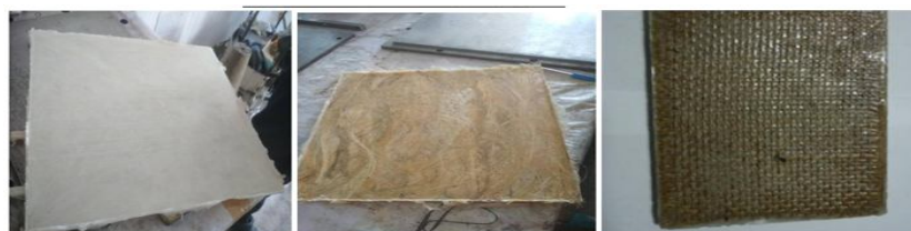
Fig.2.2.3 cotton ,sisal jute natural fiber composite
