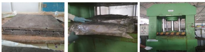
Fig.2.2.2 Placing the enclosed mould in hydraulic press
