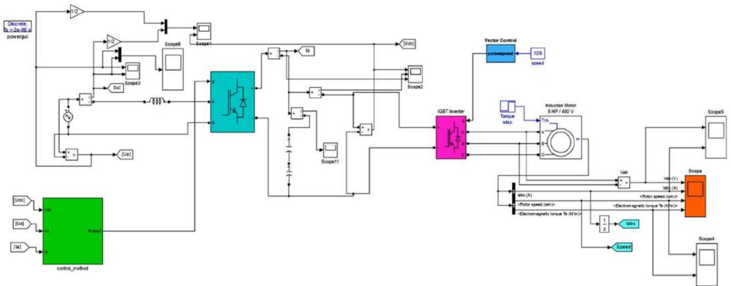
Fig 6.1 MATALB model of one rectifier system
