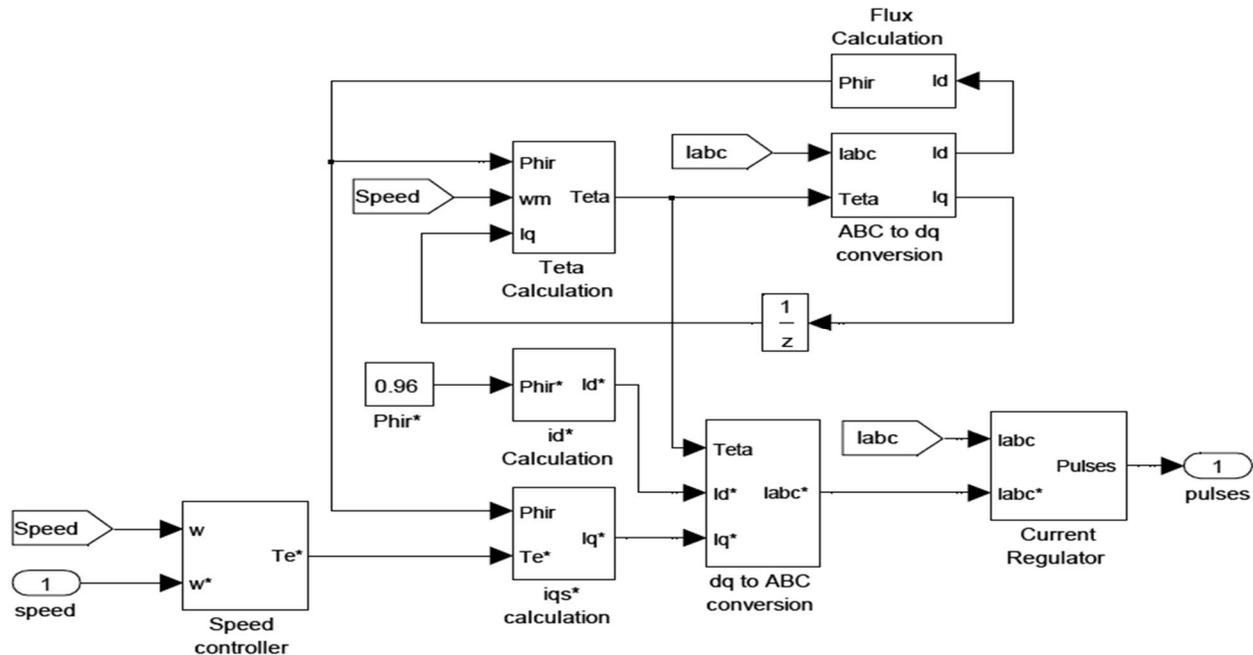
Fig 4.2: Block diagram of Vector control in MATLAB simulation.
