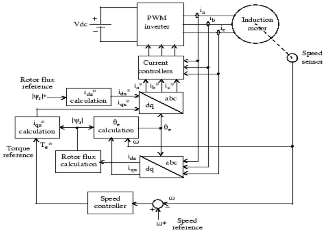
Fig 4.1: Block diagram of vector control of induction motor.
