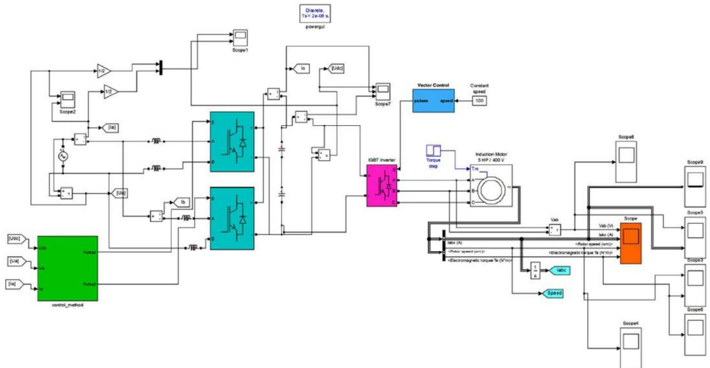
Fig 6.2 MATALB model of two rectifier system
