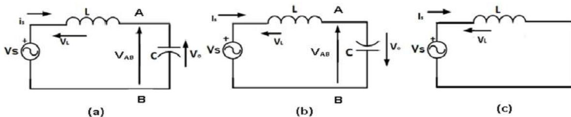
Fig 2.2: Working of Single phase PWM Rectifier Circuit
