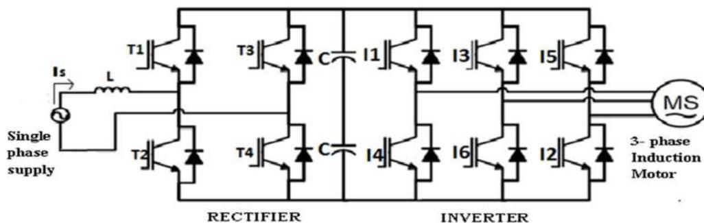
Fig 1.1: Conventional Single Phase to Three Phase Induction Motor Drive
