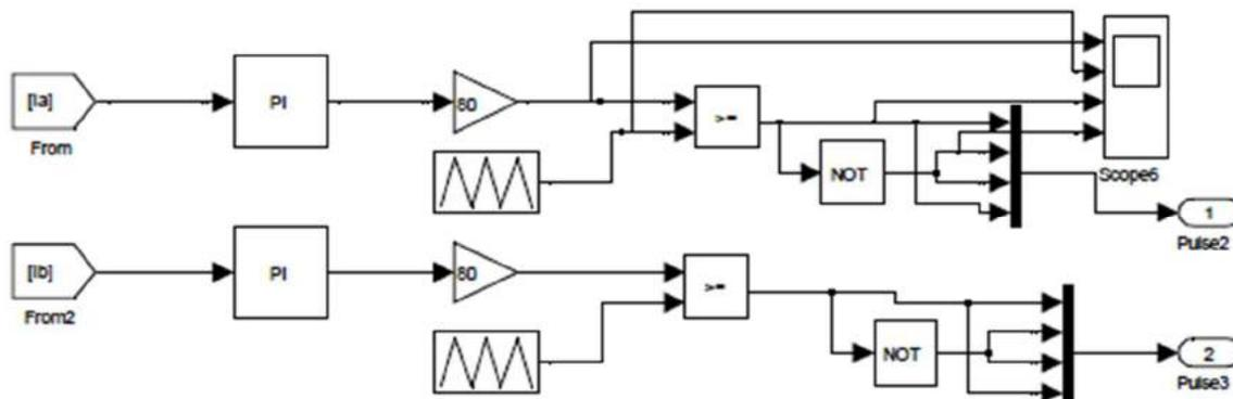
Fig 3.2: Control circuit of rectifier (part 2)
