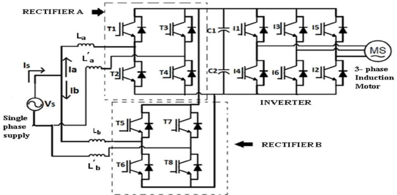
Fig 1.2: Parallel Rectifier Connected Single Phase to Three Phase Induction Motor Drive.
