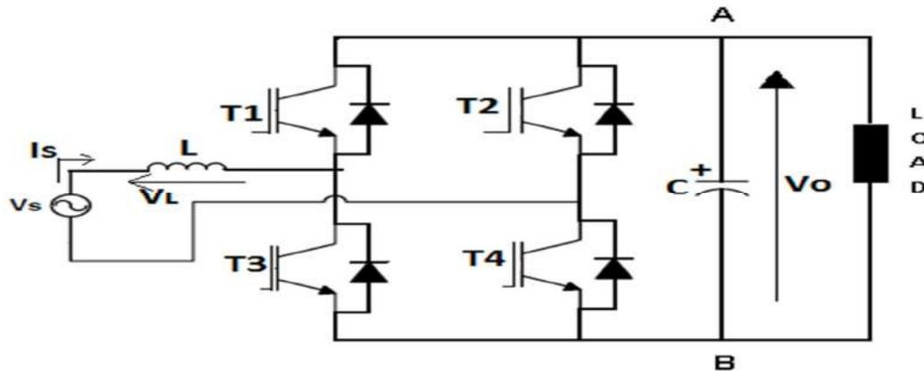
Fig 2.1: Single phase PWM Rectifier Circuit
