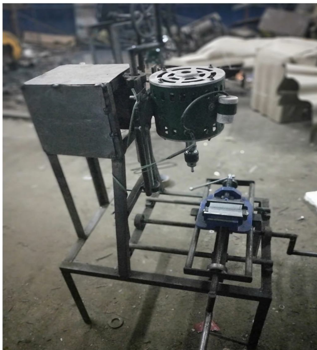
Fig 7.1 Photography of friction welding machine
