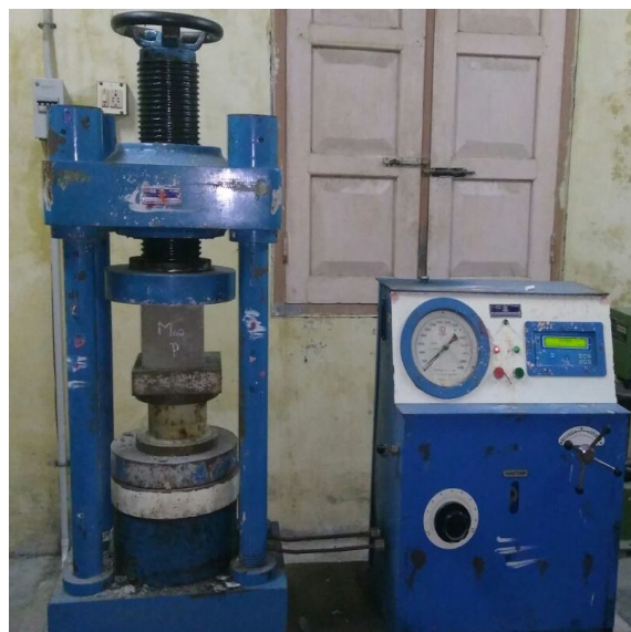
Fig.3 Compression test on concrete cubes
