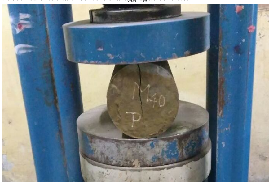
Fig.6 Failure of cylindrical specimen
