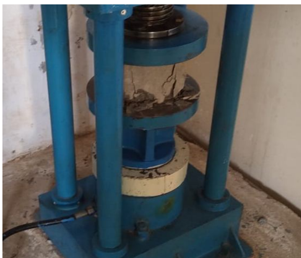
Fig.5 Failure of cube specimen
