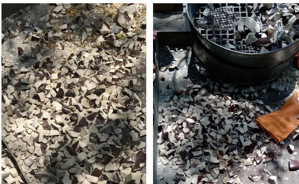
Fig.2 Crushing and Sieving of Ceramic Waste
