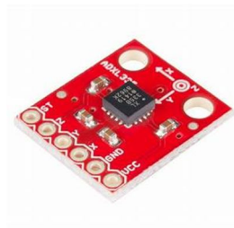
Figure 4 ADXL335 Accelerometer Sensor
