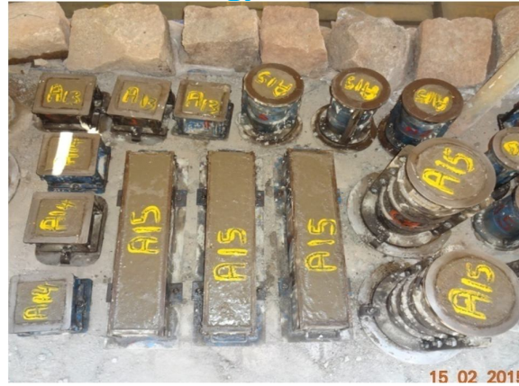
Fig 1: Moulds filled with concrete
