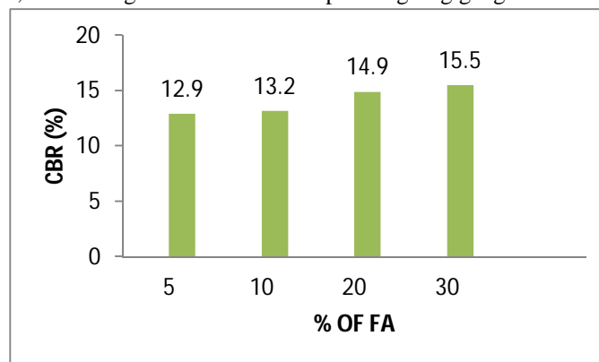
Fig 9: variation in CBR with various % of FA in unsoaked condition
