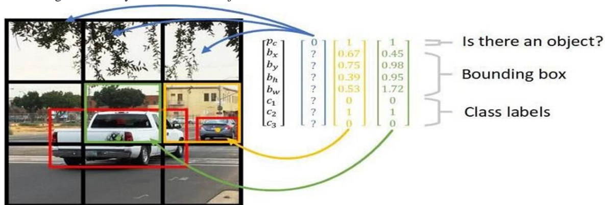
Fig 8: YOLO object detection
