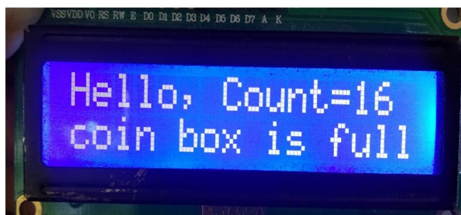
Fig 5 Message will be displayed on the display when coin box is full
