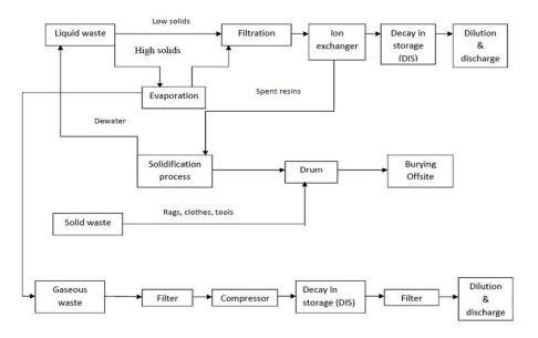
The block diagram above shows simple handling system required for radioactive waste.
