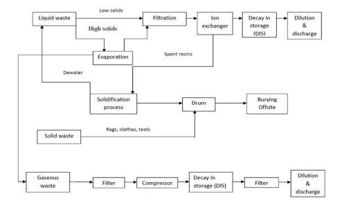
The block diagram above shows simple handling system required for radioactive waste.
