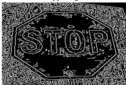
Fig4. (a). Canny detected Image with noise
