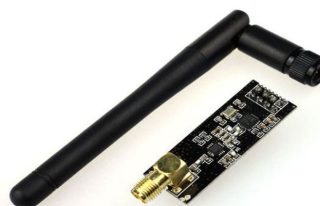
Fig 4: nRF24L01 transceiver with external antenna
