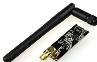
Fig 4: nRF24L01 transceiver with external antenna
