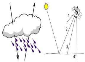
The microwave energy recorded by a passive sensor can be emitted by the atmosphere (1), reflected from the surface (2), emitted from the surface (3), or transmitted from the subsurface (4). Because the wavelengths are so long, the energy available is quite small compared to optical wavelengths. Thus, the fields of view must be large to detect enough energy to record a signal. Most passive microwave sensors are therefore characterized by low spatial resolution.
