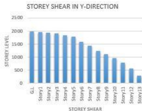
Figure 7.12 Maximum storey shear in direction of Y
