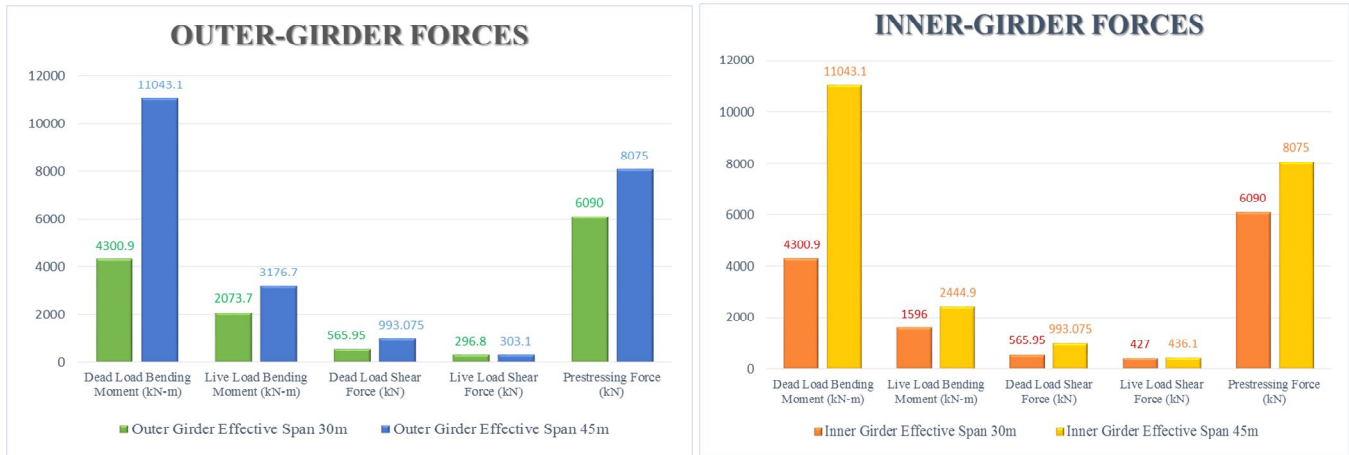
Fig. 16: Graphs indicating comparison of girder forces
