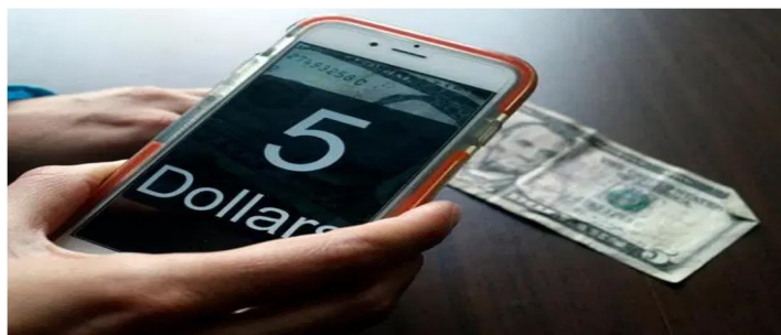
Fig.2. An example of AT that helps the user identify the currency and denomination.
