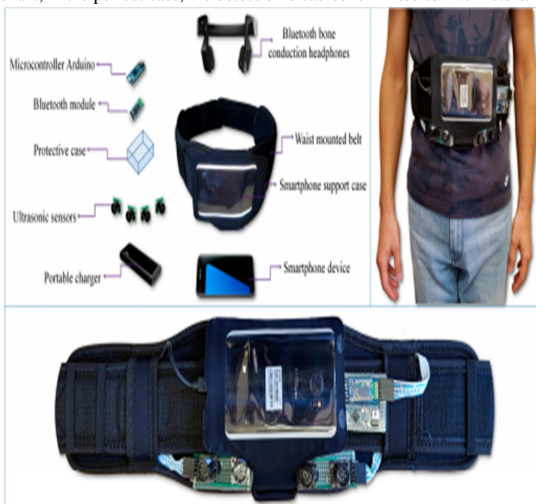
Fig.5. Combination of Ultrasonic Sensors and Computer Vision for Obstacle Detection
