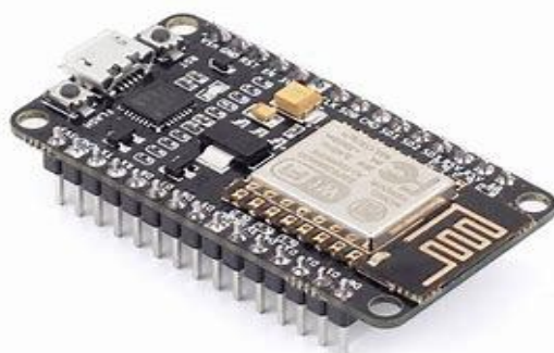
Fig 3.2 Node MCU Development Board
