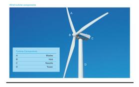
*a) Blades*: Lifts and rotates when wind is blown over them, causing the rotor to spin. Most turbines have either two or three blades. *b) Hub*: In simple designs, the blades are directly bolted to the hub and hence are stalled. The hub is fixed to the rotor shaft which drives the generator directly or through a gearbox.
