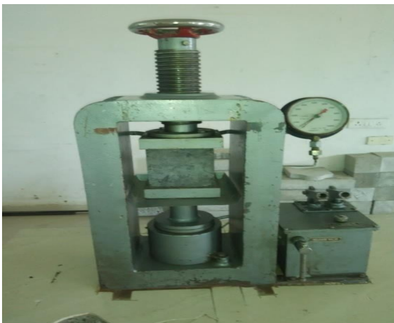
Fig. 1: Compressive Testing Analysis of Cube
