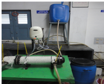
Fig. 6 Apparatus of Shell and Tube heat exchanger
