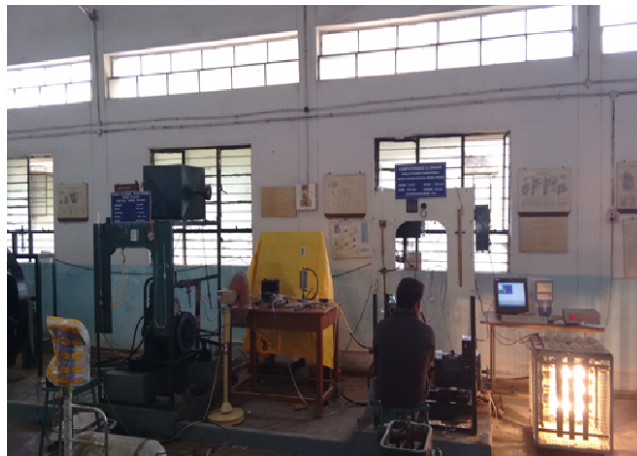
Figure II-2: Computerized, Electrical loading single cylinder four stroke CI engine converted to Dual fuel mode with CNG used as a fuel
