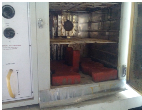
Fig. 2 Paver blocks in oven
