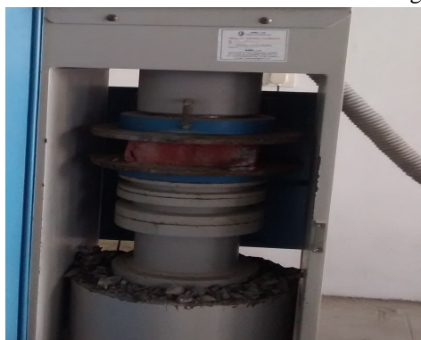
Fig. 3 Compressive strength test
