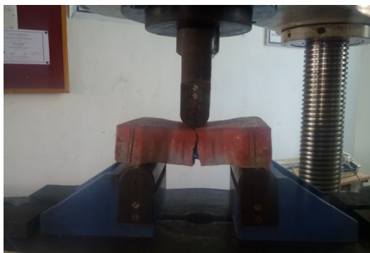
Fig. 1 Flexural strength test
