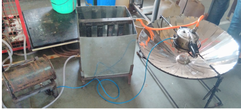
Fig. 1 Fabrication of Solar Absorption Refrigeration System
