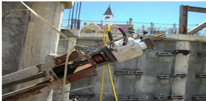
Figure 4: Testing of ground anchor
