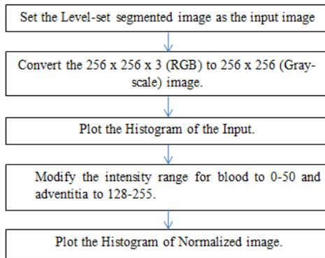
Fig.3 Flowchart for Normalization
