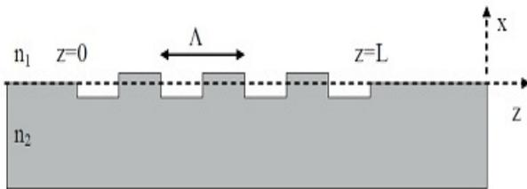
**Figure 1:** Periodic corrugation in one of the core-cladding interfaces. The grating is single mode, and we make the assumption that the only significant coupling is between counter propagating guided modes
