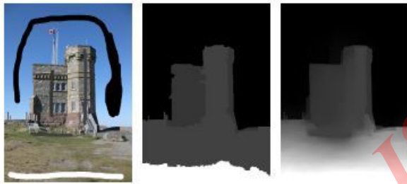
Fig. 1 The Cabot Tower example along with associated labelling and depth maps (a) Labelled Image (b) Graph Cuts (c) Random Walks.
