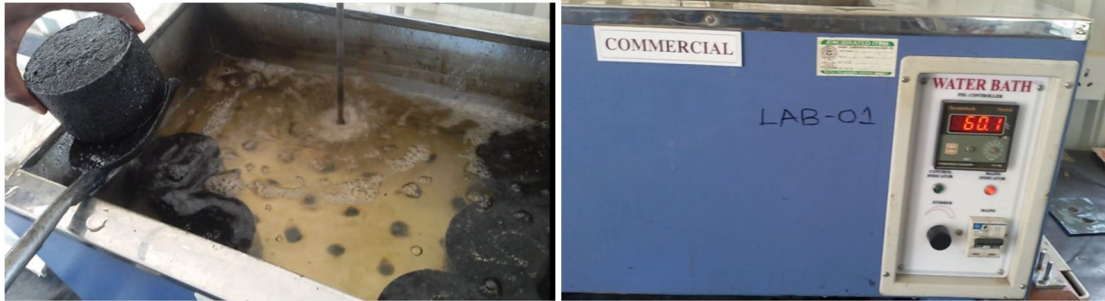
Fig 3: moulds immersed in water bath for 24 hours
