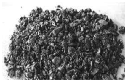
Fig 2: Loose mix(uncompacted) for air voids calculation
