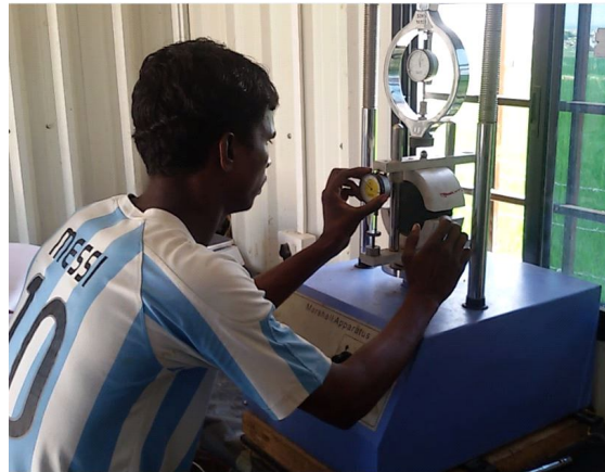
Fig 4: Marshall Stability Test Setup
