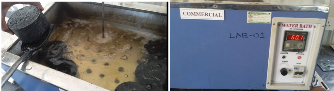
Fig 3 :moulds immersed in water bath for 24 hours
