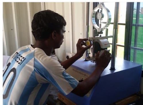
Fig.5: Marshall Stability Test Setup
