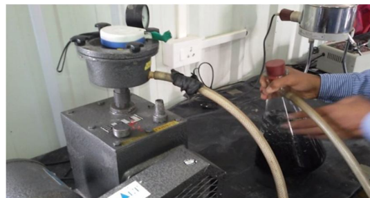
Fig.4: Air Voids determination setup
