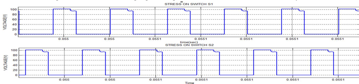
Fig.11 Simulation results of Output Voltages at S_1 and S_2
