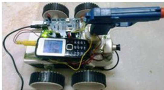
Fig.8: Implemented GSM controlled vehicle
