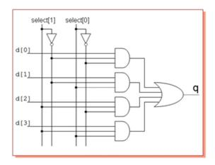
The problem that will occur while processing the Timer display will be the data lines present in the display. Since, totally 16 Data lines are present but the output obtained will be of only 8 Data lines. A multiplexing technique is used were the high number of inputs given are combined with similar Data inputs and from that a multiplexed output is obtained, that output data is sent to both the Display present
