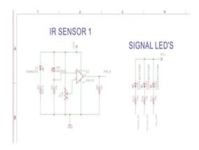
IR Sensors are used to detect any object that passes through the continuous beam of rays emitted .the detection occurs only through the perpendicular direction. The signal LED s is used to notify the lights of colours which has different purpose of its own. The Green represents the vehicle can move, Red represents stop and Yellow represents ready.
