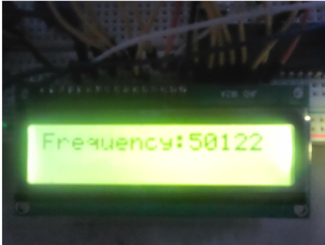
Fig. 5: Frequency output using P89V51RD2 microcontroller
