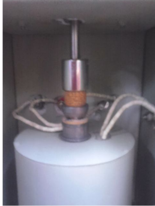
Fig. 3: Dielectric cell with PZT sample
