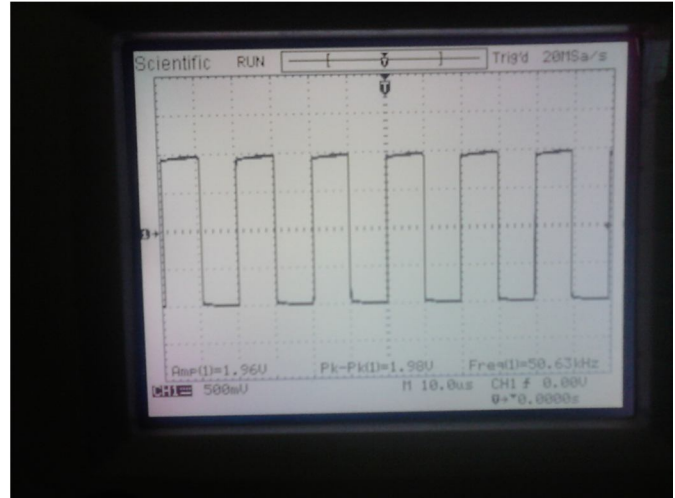
Fig.6: Frequency output using Digital CRO
