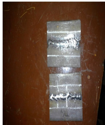
Fig-2:-Indicates welded tig and arc metal plates
