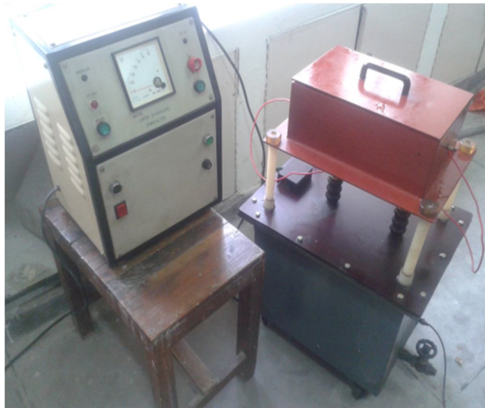
Fig-1: Solid insulation BDV experimental laboratory set-up.
