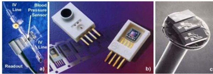
Figure (3) Disposable blood pressure sensor connected to an IV line ,(b) disposable blood pressure sensors (as shipped) , and (c) intracardial catheter-tip sensors for monitoring blood pressure during cardiac catheterisation, shown on the head of a pin.
