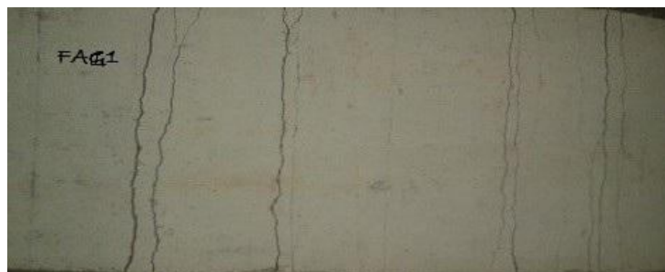
Figure 5.2 evenly distributed crack pattern in FCCG
