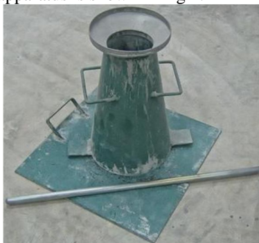
Fig 4.1 Slump cone apparatus
