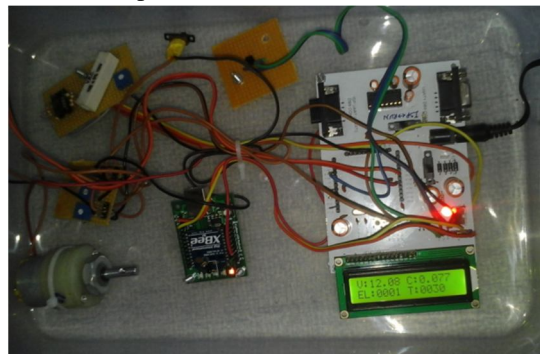
Figure2.2: Hardware used for Designing battery monitoring system
