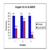
Sample 1 : 90% Cu 10%  $Al_2O_3$ Sample 2 : 80% Cu 20%  $Al_2O_3$ Sample 3 : 70% Cu 30%  $Al_2O_3$
