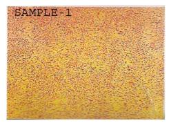
The matrix shows completely fine transformed beta as the matrix. Some equi-axed alpha also present in the matrix of beta. Microstructure of  $Cu-Al_2O_3$  at 80%-20%
