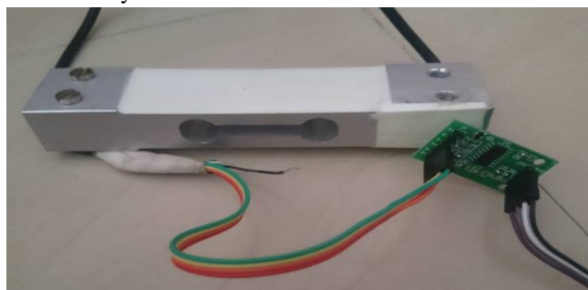
Fig. 4. Strain Gauge Load Cell
