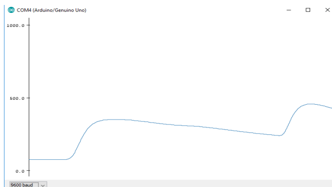
Fig. 11. MQ-6 sensor detecting gas leakage in ppm vs time
