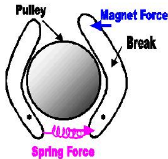
Figure 3. Diagram of the break system
