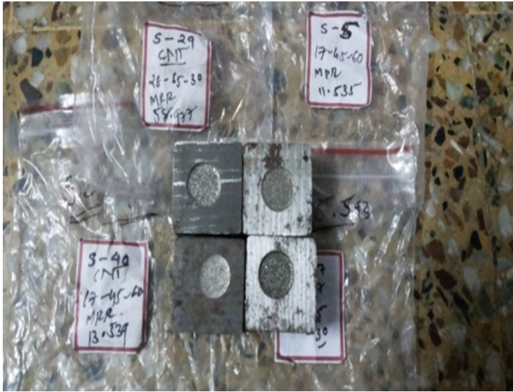
Fig 3 experiment specimen by EDM Machine
