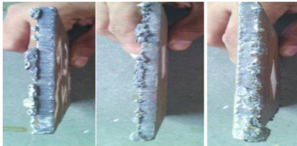
Fig.1 Gas cutting by LPG but good finishing not obtain [3]
