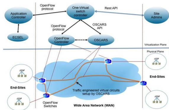
Figure 3: End-to-end virtualization using One-Virtual-Switch, ECSEL and OSCARS
