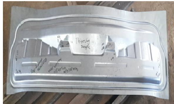
Fig.6 Actual component formed after tryout
