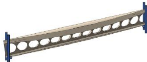
Fig 2. Lateral torsional buckling mode of cellular beams
