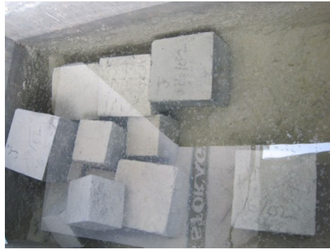
Figure. 1 Curing of Concrete Cubes (Mix+Nano-carbon Fibre)
